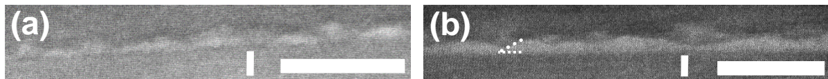
Figure 2. Cross-section high-angle annular dark-field imaging in scanning transmission electron microscopy mode of one QD plane (bright contrast) buried in an \text{Al}_x\text{Ga}_{1-x}\text{N} (0001) matrix (with x \sim 0.6 ) for a QD nominal composition of: a) \text{Al}_{0.1}\text{Ga}_{0.9}\text{N} and b) \text{Al}_{0.2}\text{Ga}_{0.8}\text{N} . The thick horizontal white line and the thin vertical one in (a) and (b) represent a scale of 20 nm and 4 nm, respectively.. The angle formed by the dotted segments between a facet and the base of a QD in figure (b) is found to be \sim 30^\circ .
